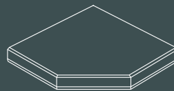
| AF 50/GetaCore® | one piece corner top angled-front-edge 1050 x 1050 x 610 x 49 mm
